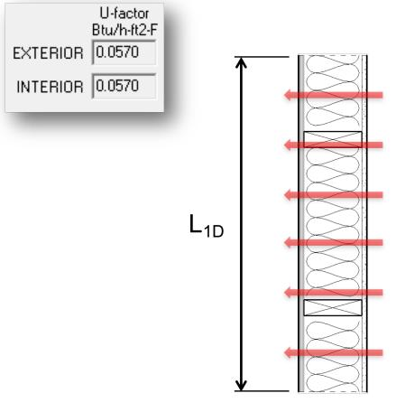
We also need to model the typical 'clear field' assembly without the disrupting element in a separate THERM file to calculate its U-Factor.
