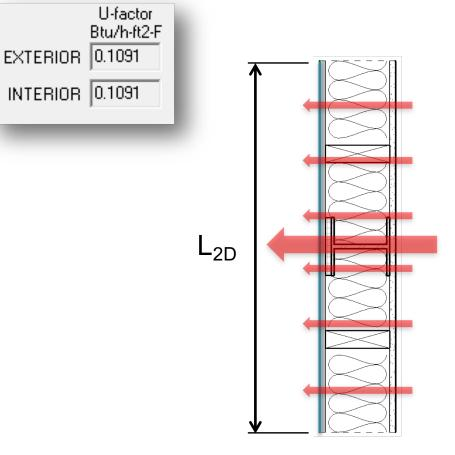
THERM's U-Factor takes into account all the particulars of the actual detail and combines it into one value which represents heat flow over the entire area
