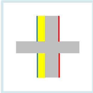
full or partial penetration of the insulating layers by materials with a different thermal conductivity
